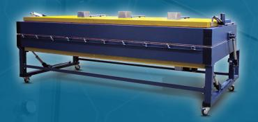
These self contained, all in one ovens, mean that producing laminated glass is now as simple as pressing a button. Using EVA film for the interlayer (any manufacturers EVA can be used), simply load the cart, and press start. EVERYTHING ELSE IS DONE FOR YOU
