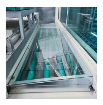
The finished laminated glass coming out of the autoclave should also be checked for suction marks, fingerprints or other imperfections. Since normal hall lighting is not helpful for such a check, a manual check can be carried out in a dark room inspection cabinet.
